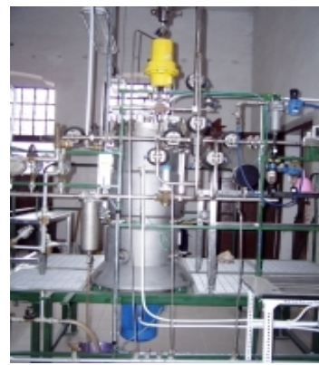
160 litre medium lab scale applied research fermentor
